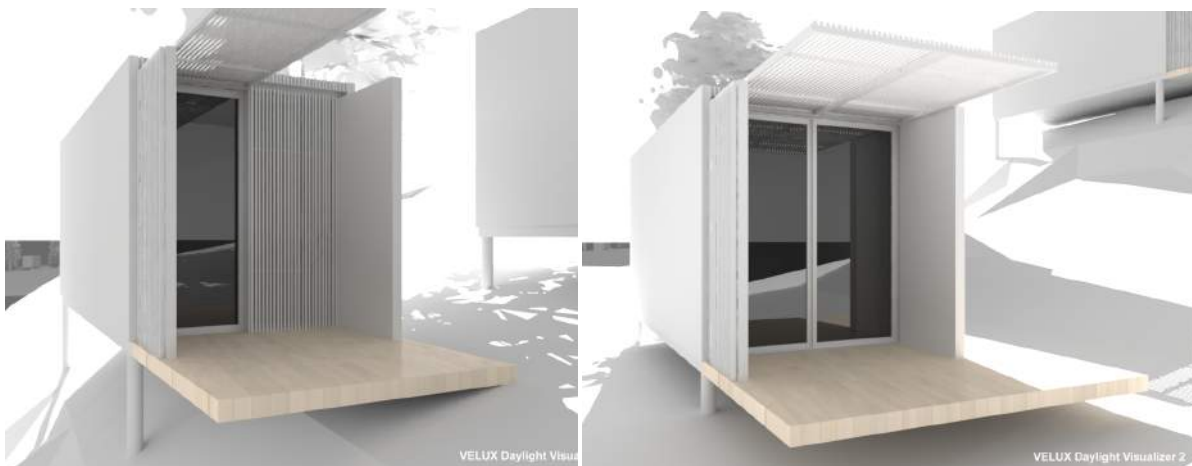
Figure 33 - Shading device used in different occasions and different ways and additions to the module, as people get more money or have other needs. A deck also helps access to the house and space to sit outside when the ground is not flat or the module needs to be set on columns.
