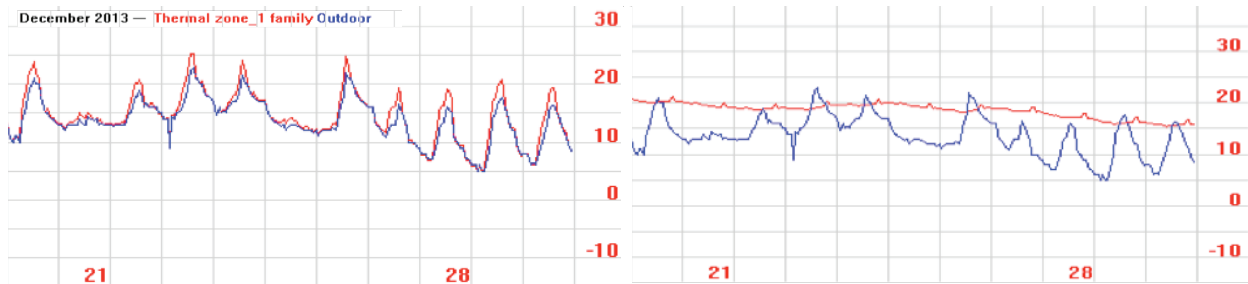
Figure 4.12 - Transmission values for container in. Riyadh, Saudi Arabia (Left) Only steel material.(Right) Steel container with 2 cm insulation on walls . The red colour represents the inside and it is clear the temperatures are a lot more balanced due to the insulation (Source: Mafalda Melo Oliveira, 2014 , based in simulation in Bsim)
