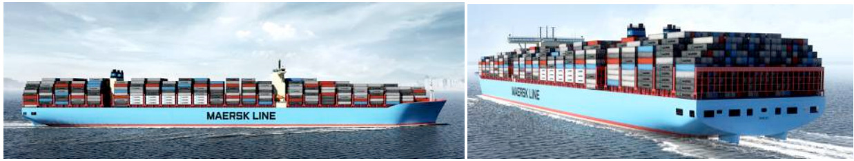
Figure 1.16 – Maersk (and World’s) biggest container boat, Triple E has a capacity of 18 000 TEU. Triple E stands for Efficiency, Economy of Scale and Environmental improved. A lot of houses would be given to a community if the boat would transport some housing units among other common shipping containers with goods. (Source: http://www.maerskfleet.com/#vessels/Maersk_Line/Triple-E )
